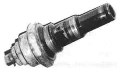
Fig. 1 Deposits on a hydraulic valve
