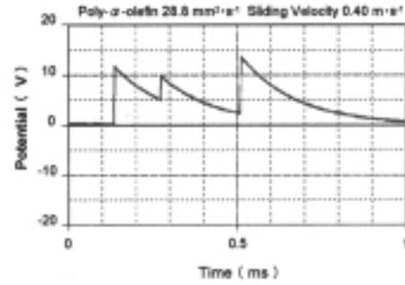
Fig. 12—The pattern of electric discharge measured at microsecond range.
