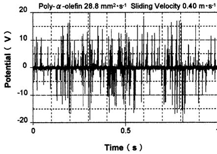
Fig. 2—The measured potential pattern without diode.
