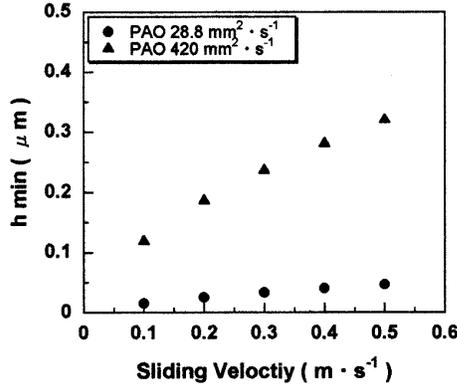
Fig. 6—The oil film thickness based on the two dimensional EHL theory vs. sliding velocity (PAO).
