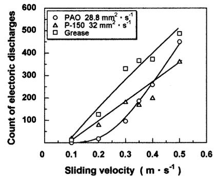
Fig. 16—The counts of electric discharges of two low viscous oils and grease vs. sliding velocity.
