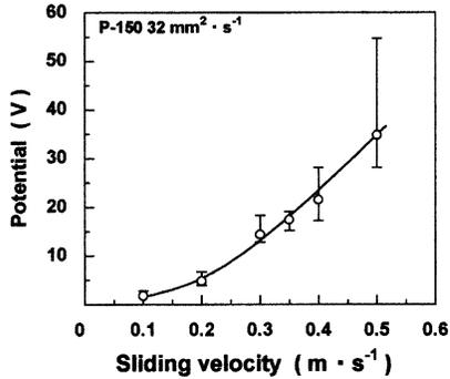
Fig. 13—The potential of hydrogenated paraffin base oil vs. sliding velocity.
