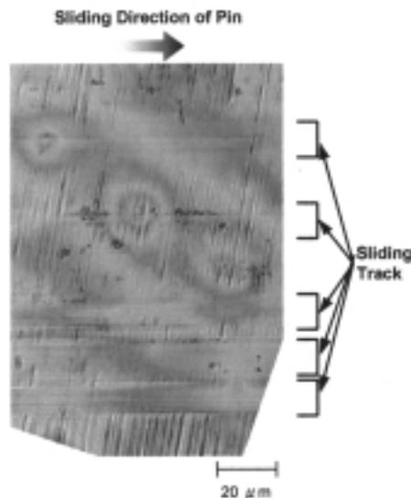
Fig. 11—The sliding track of the ball on the disc lubricated with 420 mm<sup>2</sup>/s PAO at the sliding velocity of 0.4 m/s.
