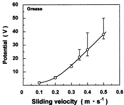
Fig. 14—The potential of grease vs. sliding velocity.
