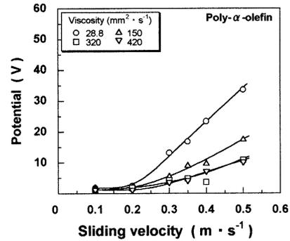
Fig. 4—The summary of the measured potentials vs. sliding velocity (PAO).
