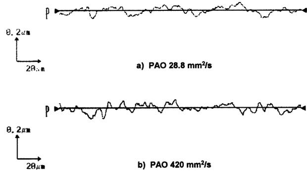
Fig. 9—The surface roughness of the sliding track (PAO).
