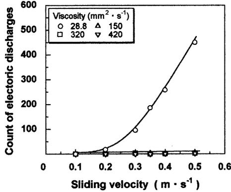
Fig. 7—The count of electric discharges vs. sliding velocity (PAO).
