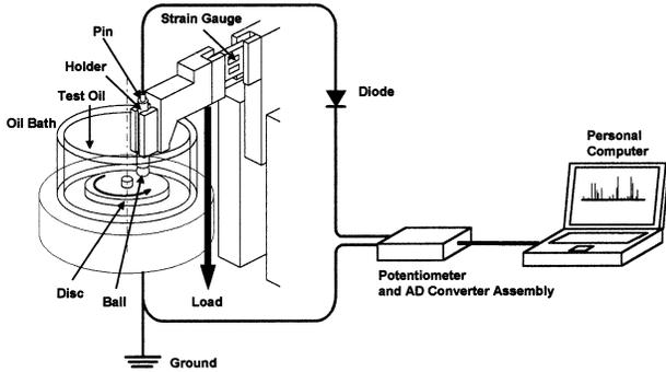
Fig. 1—Schematic diagram of test device.
