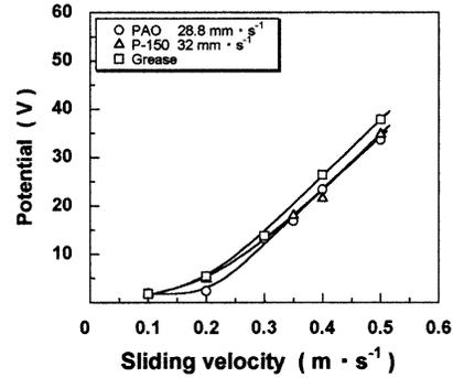
Fig. 15—The potentials of two low viscosity oils and grease vs. sliding velocity.
