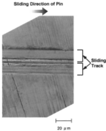
Fig. 10—The sliding track of the ball on the disc lubricated with 28.8 mm<sup>2</sup>/s PAO at the sliding velocity of 0.4 m/s.
