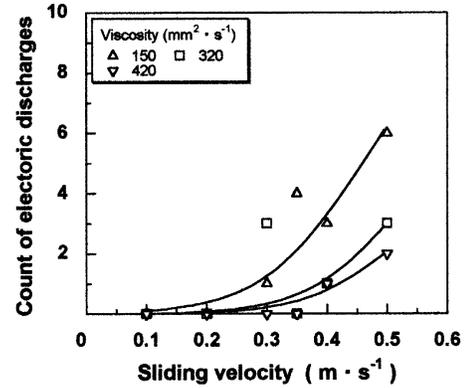
Fig. 8—The count of electric discharges vs. sliding velocity for high viscosity oil (PAO).
